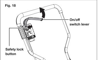
3. To stop the mower, release the On/Off switch lever.
