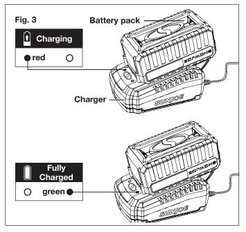
4. When the charger light turns green, the battery is fully charged (Fig. 3).
