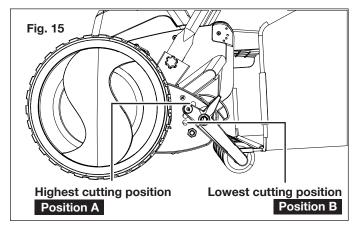
4. Other cutting heights are achieved by moving the adjustment knobs to the settings between the highest and lowest positions. Refer to the mark beside the height adjustment knobs when adjusting the cutting height (Fig. 16).
