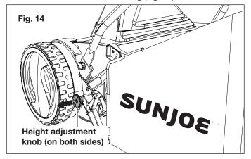
3. To adjust the reel to the highest cutting position, place the adjustment knobs through the top hole (position A) located on the sides of the reel mower frame. To adjust the reel to the lowest cutting position, place the adjustment knobs through the bottom hole (position B) located on the sides of the frame (Fig. 15).
